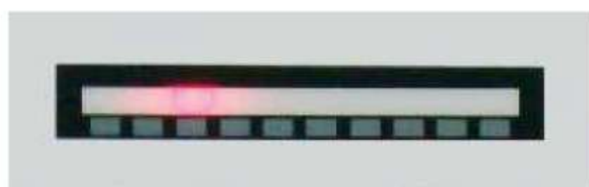
LED断针位置指示灯 LED broken needle position lamp
