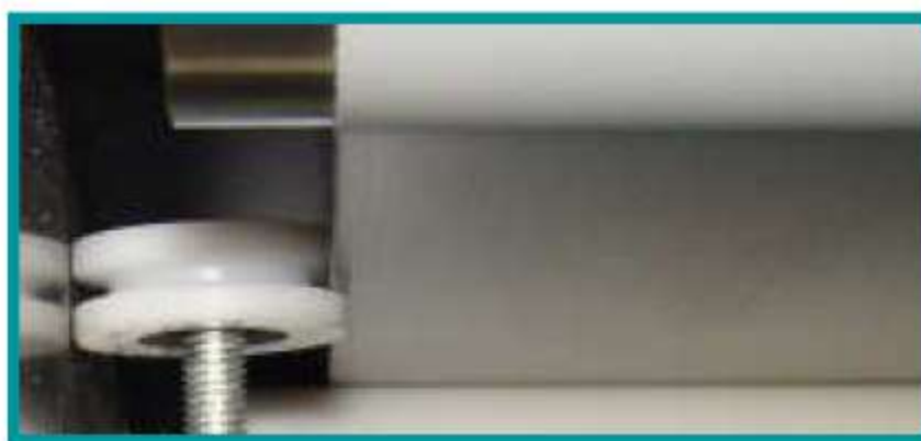
自动输送防偏保护装置 Protective device against side running of conveyor belt
