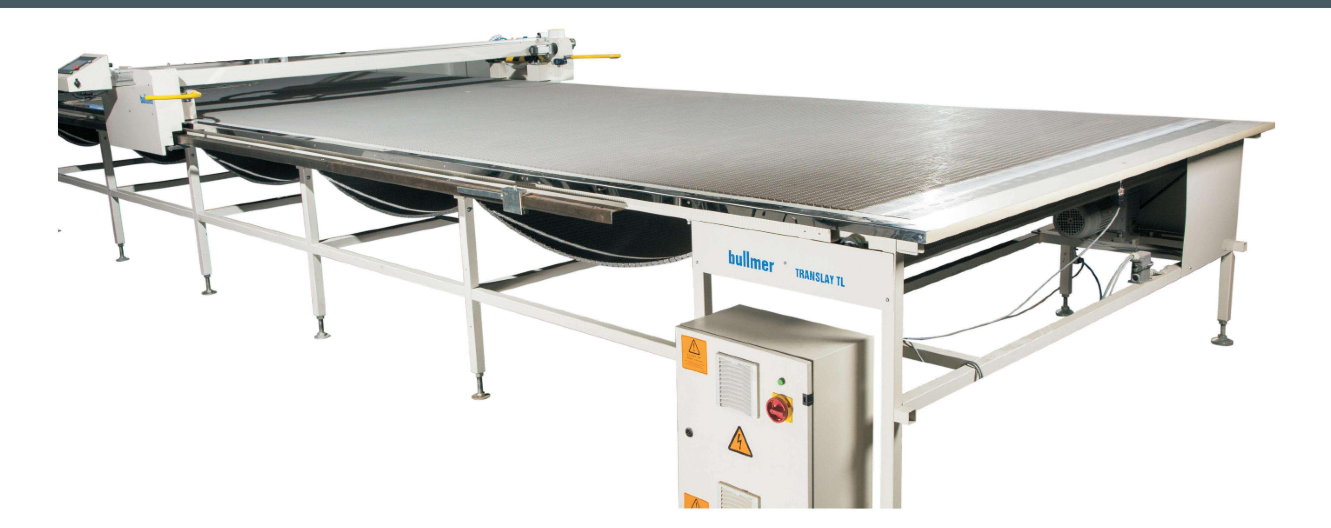
The Translay table is ideal for both knit and heavy fabric. Controlled by sensors and frequency converter, it can convey the fabric with cutter bitefeed synchronously without tension. Both auto and manual modes are available.
